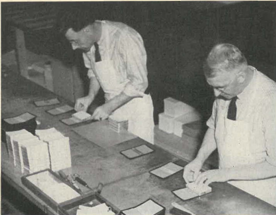
Copyrighted and used by permission SMASHED, SEWN, TRIMMED The pages are placed in the bindings.
